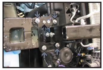
16. Slide the baseplate into position on the vehicle and start the existing 10MM (gray) and 6MM (black) hardware. Do not tighten fully. Do this on both sides of the vehicle.
