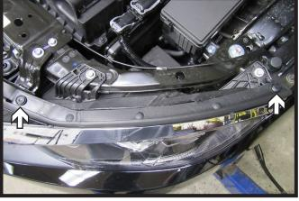
2. Remove the two (2) push pins from the corner of the chrome strip and unsnap from the vehicle. Do this on both sides of the vehicle.
