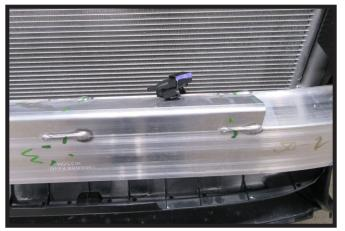
7. Remove the temperature sensor from the bumper and set aside.
