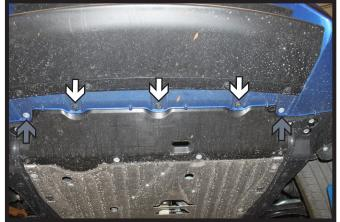
4. Using a 10MM socket, remove the bolt (gray) from the underside of the fascia. Then remove the two (2) push pins (left photo). Do this on both sides of the vehicle. Using a T30 Torx, remove the two (2) bolts towards the center (gray). Then remove the three (3) push pins (right photo).
