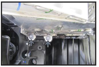
10. Using a 14MM socket, remove the four (4) bolts from the bumper (gray). There are two (2) each on the top side and underside. Using a 12MM socket, remove the bolt from the side of the bumper (white). Using a 10MM socket, remove the bolt from the top side of the bumper (black). Do this on both sides of the vehicle. Set the bumper aside it will not be reinstalled.
