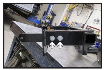
15. Place the baseplate on a flat surface and attach the support strap to the baseplate using two (2) 3/8" bolts. Make sure that the support strap is a straight as possible. Do not tighten fully. Do this for both sides of the baseplate.
