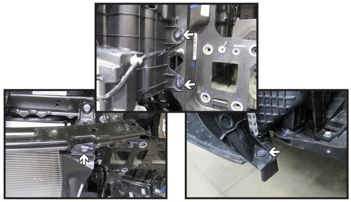
11. Remove the plastic shielding from the vehicle by removing the four (4) push pins. There is one (1) on top, two (2) along the side and one (1) at the bottom. Do this on both sides of the vehicle. The shielding will not be reinstalled.
