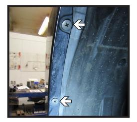
3. Using a Phillips screwdriver, remove the two (2) screws from the edge of the wheel well. Do this on both sides of the vehicle.
