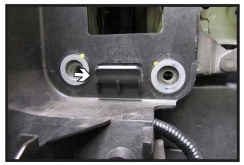
12. Using a reciprocating saw, trim the hook at the lower bumper bolt location flush with the frame. Do this on both sides of the vehicle.
