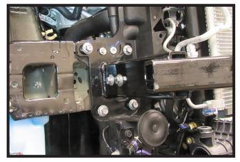
18. Start to remove each bolt that attaches the baseplate to the frame individually and apply Loctite Red and reinstall bolt and tighten to the appropriate torque. Use the following order to remove the bolts individually:10MM, 6MM, 5/8", then finally the 3/8" bolts attaching the support strap.
