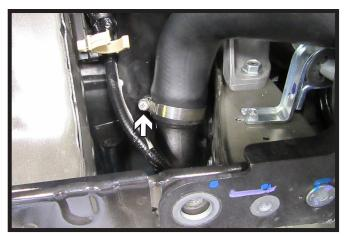
14. Using a 10MM socket remove the bolt attaching the clamp to the turbo air coolant tube.
